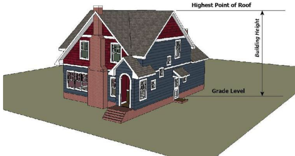
Figure 1111-G: Measurement of building or structure height
